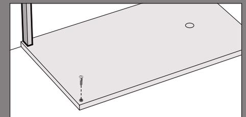
9. Apply a fine bead of the supplied silicone around the locating disc and then position the fixed panel assembly into its compensator and over the locating disc.
