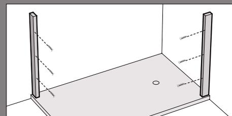
6. Re-fit the doors 'dry' and recheck the levels and contact of the seals on the tray. To plot the position for the correct placement of the fixed panel, mark centre lines at the bottom of the vertical support post on the corner.
