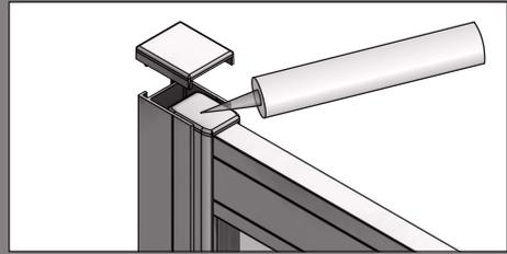
25. Ensure all non-moving parts are sealed with the silicone supplied, i.e. compensators inside and out. Ensure the bottom of the rise and fall hinges are significantly sealed with silicone.
