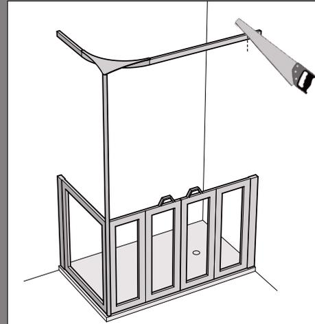
NOTE: When connecting the rail using the boomerang bracket, some care must be employed to ensure that the post remains plumb to 90°. An undersized or oversized rail will pull or push the post off the plumb, which can have a negative bearing on how the door closes and seals with the magnetic retainer.
