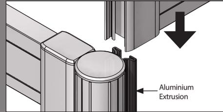
2. Set up the enclosure on the tray or wet floor. Ensure that the enclosure forms a perfect right angle and that the door seals are sitting fully on the seal platform of the tray, then mark the position of the compensators on the wall with a pencil.
