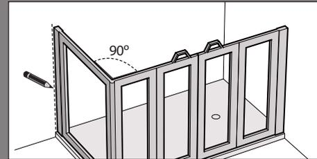
3. Using a spirit level, ensure both compensators are vertical 90°, and mark the position of the compensators' locating slots on the wall panels/tiled walls with a pencil.
