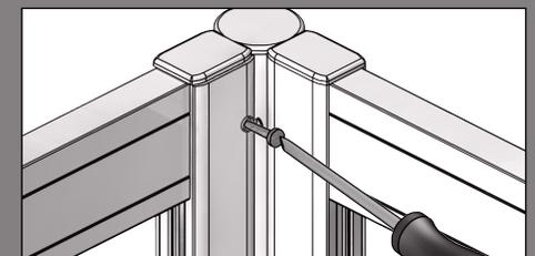
11. Slot the top half of the vertical support post over the square locating peg and secure the post in place using 2 of the 3.5mm x 22mm screws and 2 screw cap covers.
