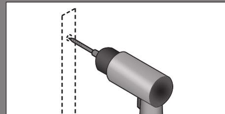
5. Using 6 of the 3.5mm x 35mm pozidrive fixing screws supplied, realign compensators and drive screws home ensuring compensators are vertical 90°.
