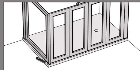
7. Remove the doors and extend these centre lines to mark a centre spot and then drill a pilot hole with the supplied 3mm drill bit.
