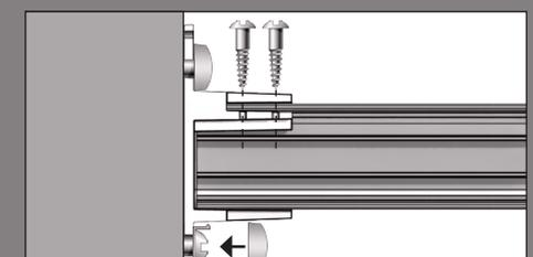
24. Apply a small amount of silicone to the top of each door between the compensators and snap fit the compensator caps in place.
