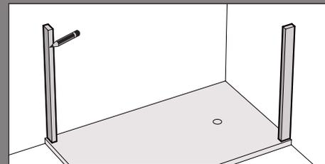
4. Using a 6mm masonry drill bit, drill the pilot holes for the compensators into the walls and then fit the 6 rawl plugs.
