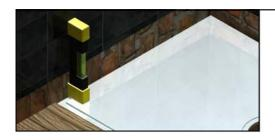
5. Re-position Flowaway® into the floor to ensure a good fit. Use a short rule or spirit level to ensure it is flush with the wall.
