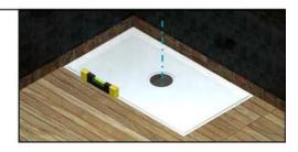
14.In accordance with the manufacturer's instructions, fit the waste system and check levels prior to leaving Flowaway® for curing - check level again with light load applied.
