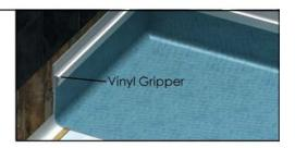
23.To finish installation, ensure wall panels or tiles are resting on the tiling lip of the cap tile strip and have been sealed along their length with silicone.
