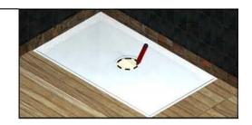
11.Cut a clearance hole in the sheeting for the McAlpine trap supplied.
