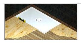
18.Sheet the area with 6mm ply up to the edge of the Flowaway®, covering the 6mm rebate.
