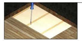
Once you are sure of the levels, secure sheets in place using suitable screws. 10.Re-position Flowaway® and check levels. Mark the position of the waste.
