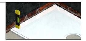
In accordance with the manufacturer's instructions, fit the waste system and check levels prior to leaving Flowaway® for curing - check level again with light load applied.
