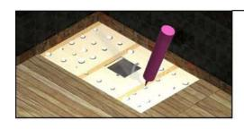
15.Bed down the Flowaway® to the joists using Pink Grip, No Nails or other suitable material.
