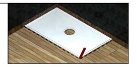
4. Using this line, cut and remove the floorboards. Identify existing waste outlet and plan waste route.
