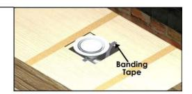
13.Re-position the Flowaway® and ensure the trap aligns with the waste position on the base.
