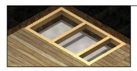
Using support batons, span the breadth of the joists to create a supporting edge for the Flowaway®, taking care not to offset levels.
