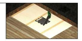
12.If necessary, secure the trap in position using banding tape from the packaging, positioning it between the joists.
