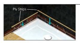
19. As the Flowaway® is not handed, strips of 6mm ply must be cut and placed on the inside edge of the unique rebate adjacent to each wall. These should be secured in place using silicone adhesive.
