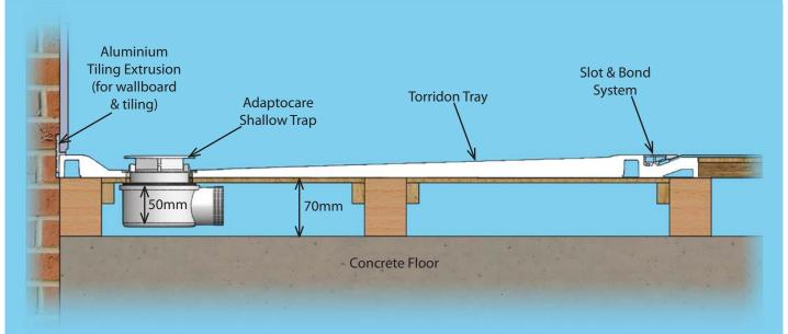
Dwanging & sheeting between the joists is recommended to provide a solid platform for the tray.
